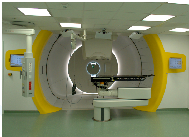
Gantry facility with a scanning proton beam for irradiation of tumours located at any site of the patient's body, except the eyeball
